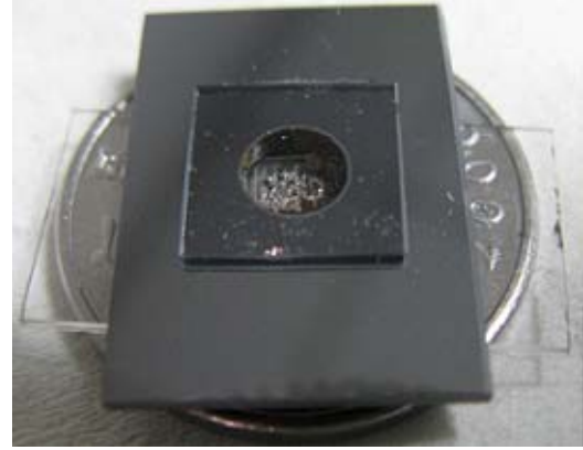
Fig. 2 Photograph of a sealed cell (10×20×1mm). Shiny Rb drops are visible.
